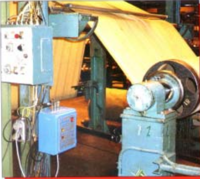
Elimination of static charge on movable material surfaces (paper, plastic, textiles etc with NO STATIC)
