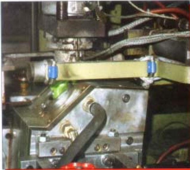
NO STATIC installed on plastic machine with adaptation at machine tool
